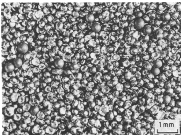
Figure 5 Photograph showing the size distribution and typical shapes of the steel balls used as the erodent in this study.
